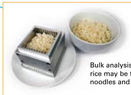
The Rice Texture Analyzer with VectorPro software performs both standard texture profiling and custom mechanical sensory measurements by use of interchangeable fixtures
