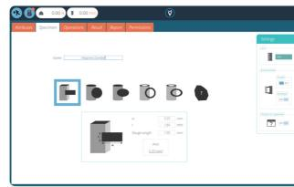
▲ Select the appropriate form of your specimen and the extensometer setting
