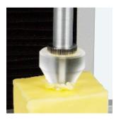
Mecmesin offers six Perspex and one stainless steel conical probes with angles ranging from 15° to 90°. Cone penetrometry is traditionally used within dairy products to assess hardness and spreadability. It has also found application in biscuits and other similar brittle products.
